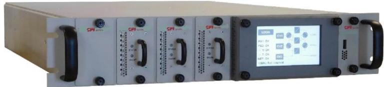
Hot-swappable, plug-in upconverter and downconverter modules
